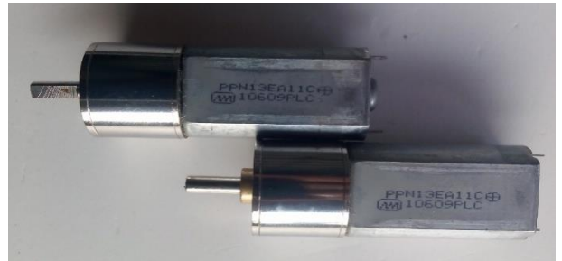
Fig.9: DC geared motor.
